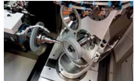
The new dressing unit on the VOLLMER 360S.
