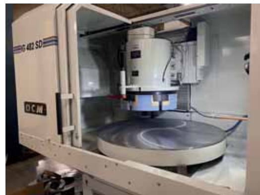
The DCM Tech IG 482 SD rotary surface grinding machine with a 1,220mm diameter.
