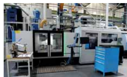
Kellenberger 100, automated with Wenger WeFlex pallet loader. Machine travels: Z-axis: 1150/750 mm, X-axis: 365 mm.
