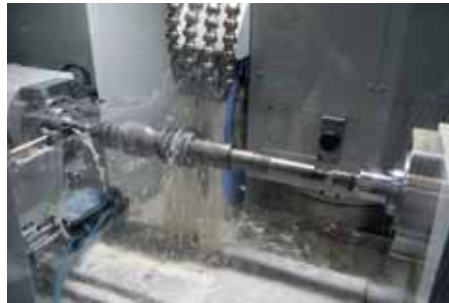
Grinding between centres of a table section screw for a Liebherr BK2 machine.
