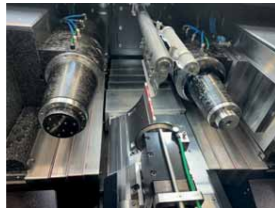
Carbon fibre spindles on the Tschudin Cube machine.
